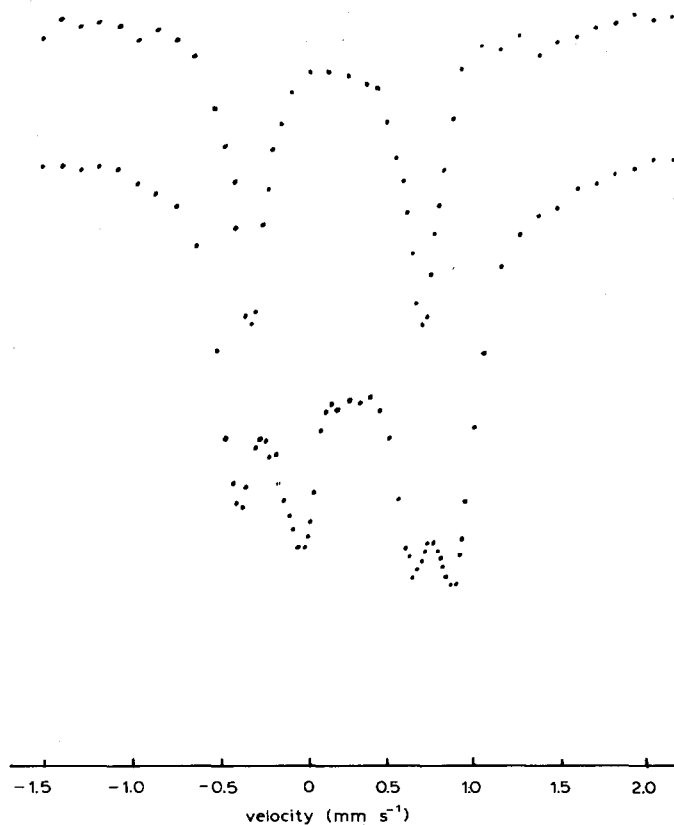
Fig. 2. Mössbauer spectra of [\text{FeRu}_3\text{H}(\text{CO})_{12}\text{N}] (IV) upper curve, and [\text{Fe}_4\text{H}(\text{CO})_{12}\text{N}] (V) lower curve.
